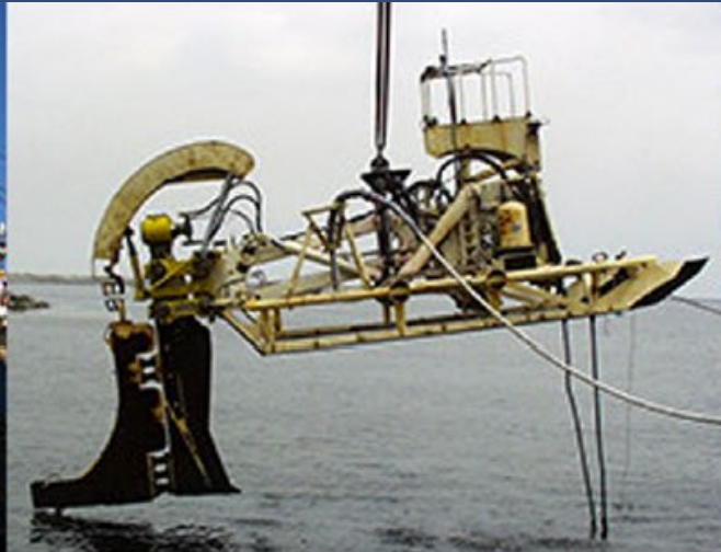
Fig. 1. Wheel cutter (left); Plough (centre) and Towed Jetting Vehicle (right) (courtesy: www.ldtravocean.com ).
