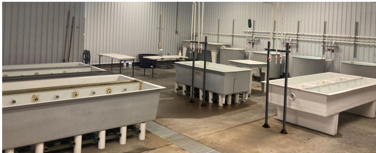
Figure 5. Photograph Hog Island Oyster Co. Humboldt Bay hatchery. Larvae tanks are located on the back wall, with upwellers and downwellers in the center and to the left.
