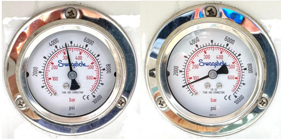
Figure 2. The hydrogen storage pressure gauge at the start and end of the Ukiah test run
