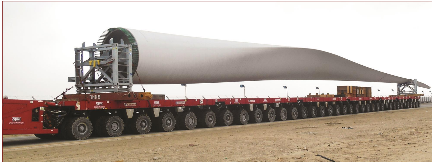
SPMT transporting WTG blade. Source: KHL Group
