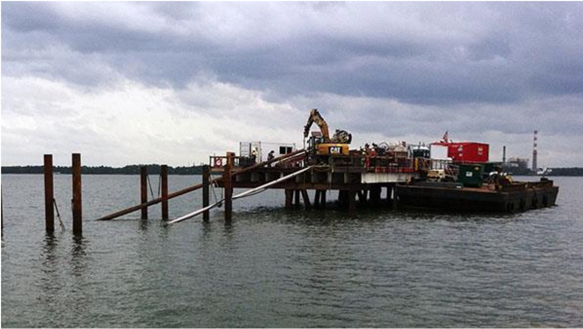
Figure 10. Example Marine Support Jack-Up Barge for an HDD
