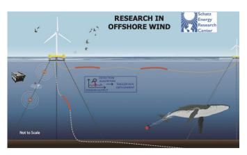
debris, while posing an entanglement risk to wildlife (i.e. secondary entanglement). Our entanglement mitigation project will develop a system of technologies to monitor and identify mooring line entanglements. We will use computational simulations to predict floating platform motions and mooring cable loading for a variety of entanglement scenarios.
