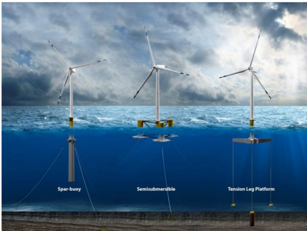
Figure 1. Floating offshore wind substructure topologies including spar-buoy, semisubmersible, and tension leg platform. Illustration by Josh Bauer, NREL.
