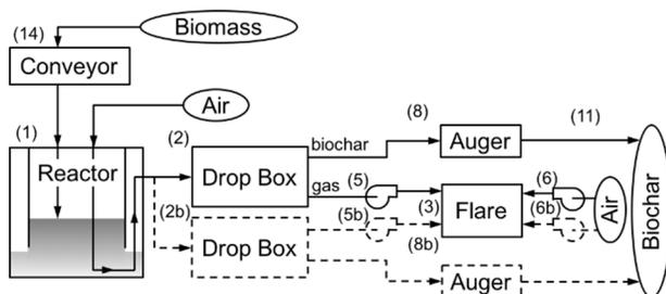
Figure 3. Simplified process flow diagram for single-auger unit (solid lines only) and dual-auger unit (solid and dashed lines). The numbers in parentheses refer to the annotations in figure 2; annotations appended with 'b' indicate additional equipment for the dual-auger unit.
