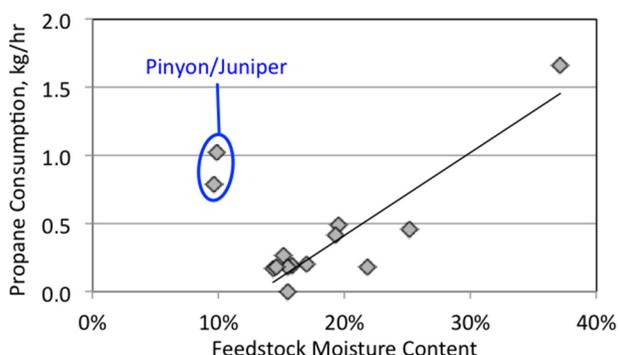
Figure 8. Propane consumption vs. feedstock moisture content on a dry basis.
