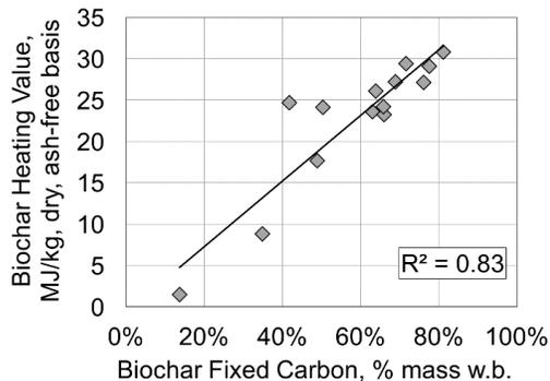
Figure 7. Biochar higher heating value on a dry, ash-free basis versus fixed carbon content.
