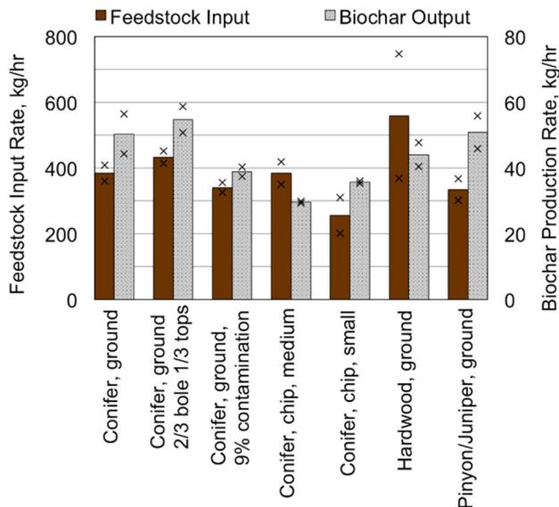
Figure 4. Average feedstock input and biochar production rates with various feedstocks. The black 'x' symbols represent the values from replicate test runs, and the height of the bar shows the average.
