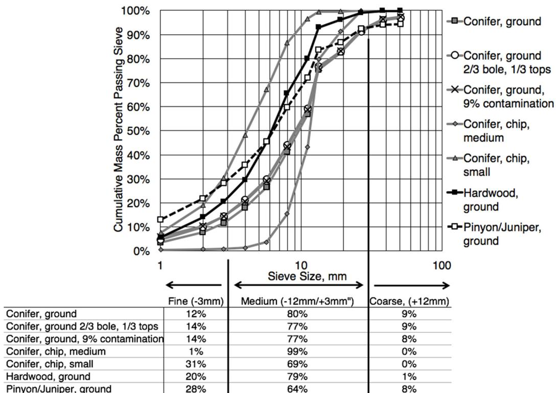
Figure 1. Cumulative particle size distribution of different feedstock mixtures plotted on a log scale.
