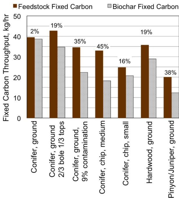
Figure 5. Fixed carbon input and output rates. The percentage value above each set of bars indicates the percent of fixed carbon lost on a wet basis.
