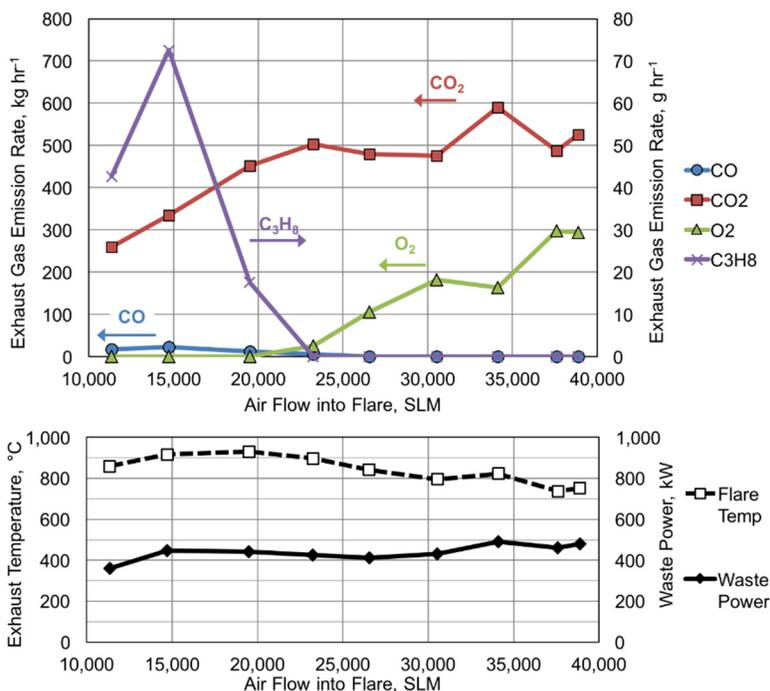
Figure 9. (a) Gas emissions and (b) temperature and waste heat from the flare with supplemental combustion air. The colored arrows in the upper plot indicate which y-axis is used with each of the respective exhaust gas concentration values.
