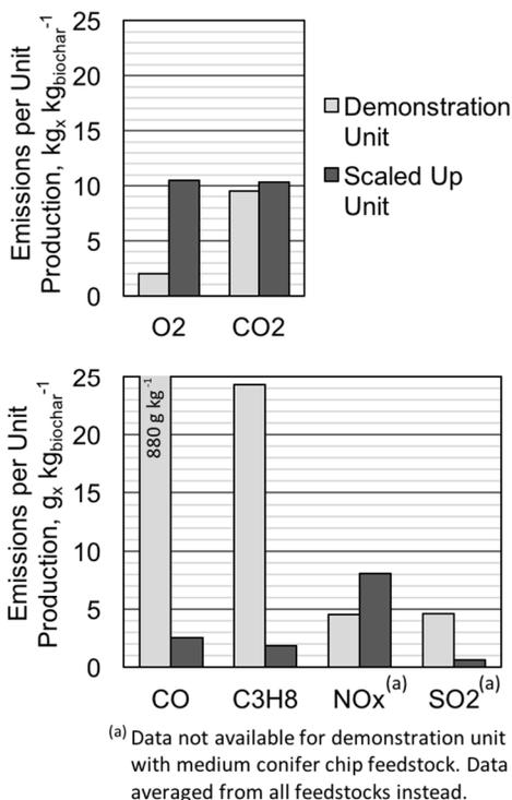
**Figure 10. Comparison of emissions averaged from all feedstock types on the single-auger unit (light bar) and both tests of the dual-auger unit (dark bar).**
