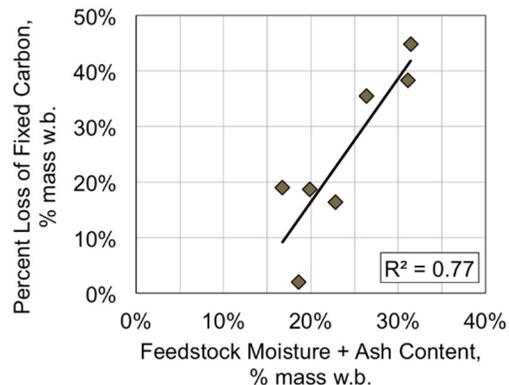
Figure 6. Fixed carbon loss versus the sum of feedstock moisture and ash content.
