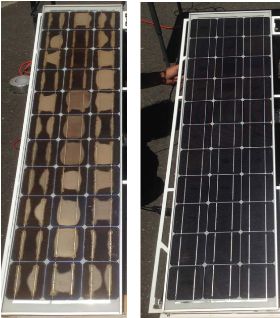
Fig. 4. A physical comparison between a 26-year old ARCO M75 module and a 19-year old Siemens SM50-H (Photos by Jake Rada)
