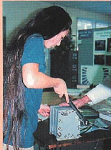
Nicole D'Arcy tightens the bolts on the fuel cell stack.
