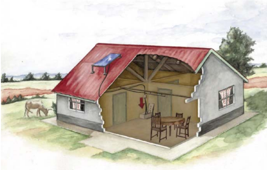
Figure 1: Solar electric system during the day. The solar module is on the roof, and a wire delivers the electricity to the battery which is located inside. An arrow indicates the flow of electricity into the battery during the day. (image by Michael Okendo)
