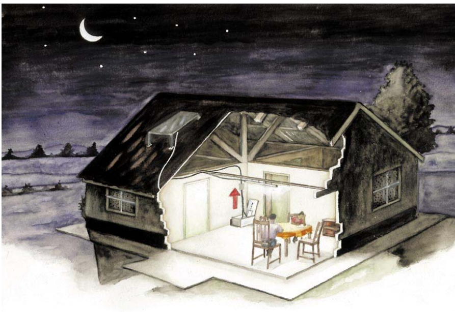
Figure 2: Solar electric system at night. An arrow indicates the flow of electricity from the battery to power the light. (image by Michael Okendo)
