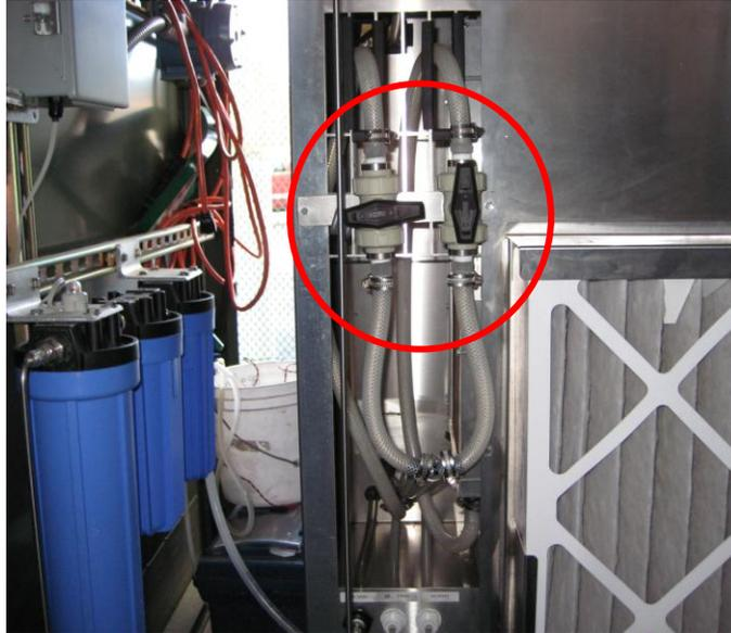
**Figure 5. Heat exchanger outlet and bypass valves installed at back of electrolyzer unit**
