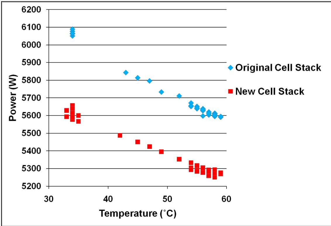
**Figure 6. Relationship between cell stack power and temperature**
