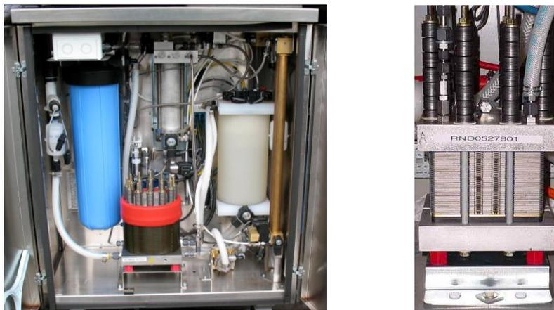
**Figure 1. To the left is Proton's original S40 cell stack installed in the HOGEN® electrolyzer at the HSU station and to the right is Proton's Next Generation Cell Stack.**
