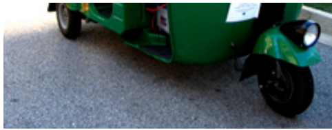
The Indian Bajaj three-wheeler single-cylinder i.c. engine taxi converted by Energy Conversion Devices from compressed natural gas fuel to hydrogen under a partnership program between the U.S. government (USAID) and industry.
