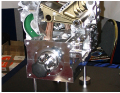
A cutaway model of the compact two-stroke engine designed by New Zealand's Pivotal Engineering Ltd. The triangular shape is the "piston" moving up and down in an arc, attached to the shaft on the right.
