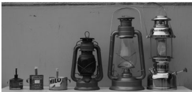
Fig. 1 An illustrative subset of the tested lamps. Left to Right: Three simple wick lamps, two hurricane lamps, one pressure lamp
