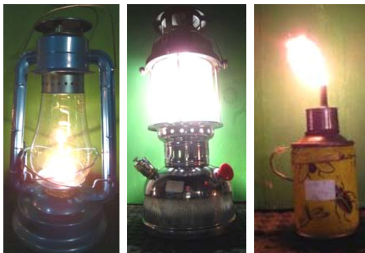
Fig. 1. Typical fuel-based lighting technology (left to right): 'Hurricane' lamp with glass wick cover, pressurized fuel lantern, and open-wick lamp made from a recycled consumer goods canister. Photos by Peter Alstone.
