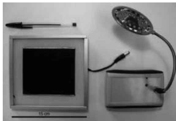
Fig. 2. Gooseneck lamp and solar module offered for sale in the study. The AC-DC recharging circuit ("wall wart") that was available as an alternative to solar charging is not pictured. The pen is shown in the picture for scale. Specifications - useful battery life: 1000 mAh, useful battery energy: 3.7Wh, lighting service duration: 10h, peak illuminance at 1 meter: 14 lx, PV power: 1W
