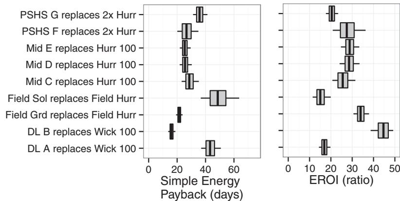
**Figure 5** Simple payback and energy return on investment (EROI) for combinations of improved lighting and fuel-based lighting being replaced (all assume a 2-year lifetime). Box plots show the interquartile range (box) and 90th percentile range (whiskers). The product descriptions that correspond to each product referenced here can be found in table 1.
