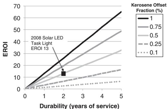
**Figure 6** Energy return on investment (EROI) for an LED lighting system with 140 megajoules (MJ) of embodied energy that is used by someone with baseline fuel use of 5 MJ/day as a function of durability (with years of service as a proxy variable) at various kerosene offset fractions (the fraction that is offset by adoption of the modern light). An example product is shown with a black square based on observations from the field in 2008. LED = light-emitting diode.
