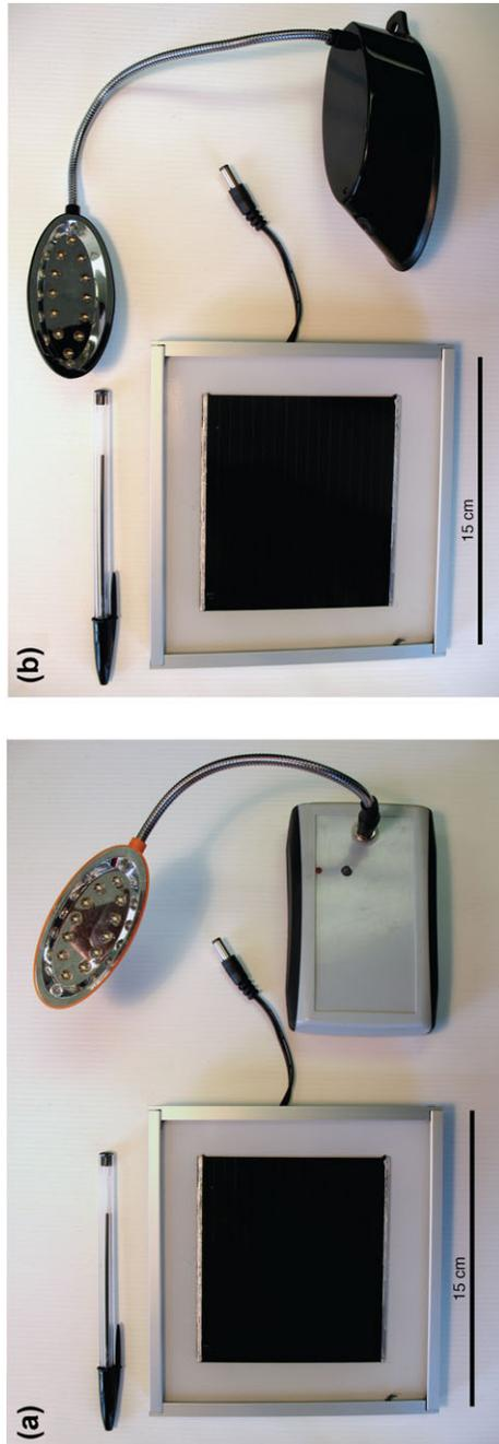
**Figure 2** (a) The gooseneck lamp we offered for sale in Kenya with a 1-watt copper indium selenide solar module. (b) A commercially available gooseneck lamp that was the basis for the lamp we sold. It has the same internal components. The pen and a 15-cm solid line are included for scale.
