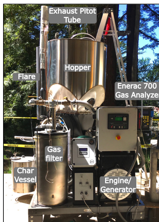
Figure 2. Photograph of the experimental set-up the All Power Labs PP20 gasifier genset.
