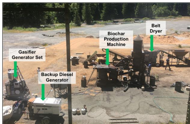
Figure 2. Picture of integrated biochar production system during steady state testing.
