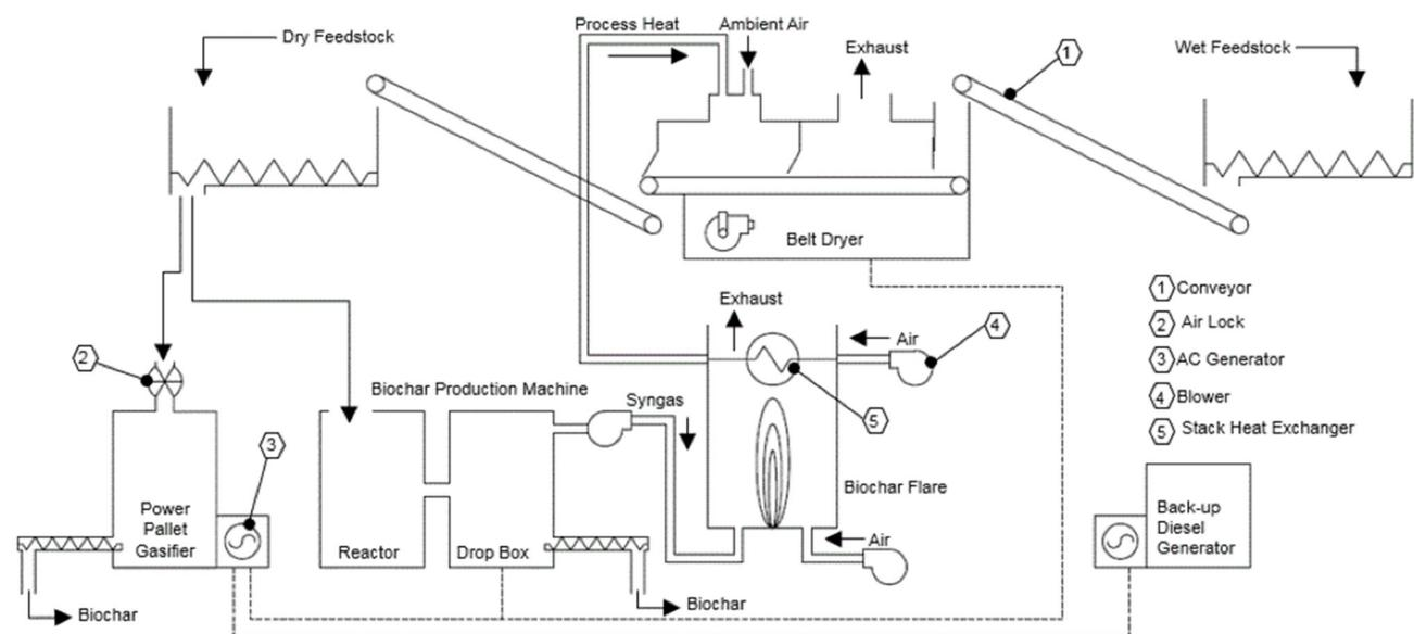
Figure 1. Simplified schematic of integrated biochar production system as tested.
